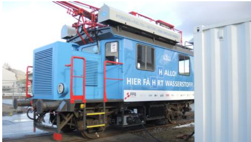
Freight Locomotive Powered by Accelera Fuel Cells. (Source: Business Wire)
