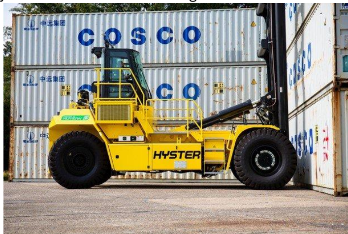
Hyster® container handler powered by hydrogen fuel cells (Source: Nuvera)
